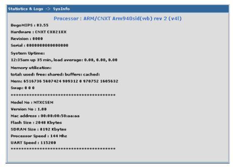
This is an example of the System Information Statistics & Logs screen. It shows the information of the module: processor details, uptime memory, utilization, version, date, binary details.
